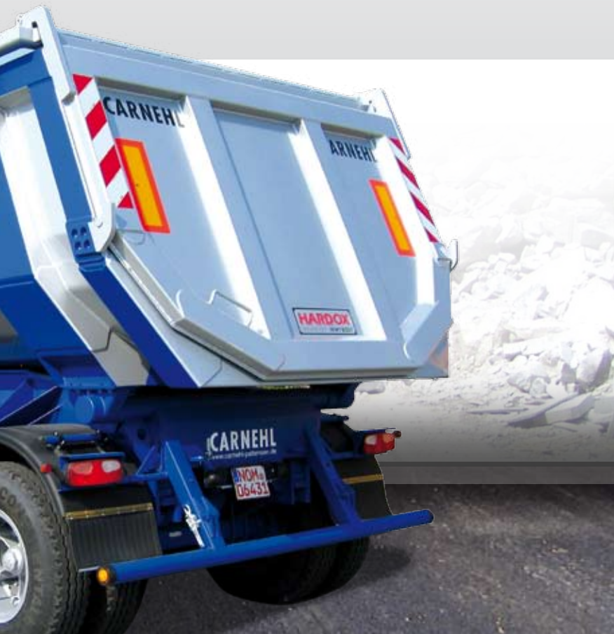
External tailgate with rectangular body end
