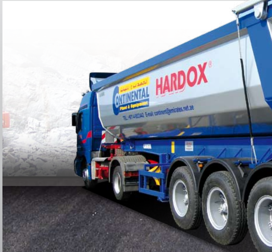
3-axle semitrailer with approx. 50 m 3 capacity
