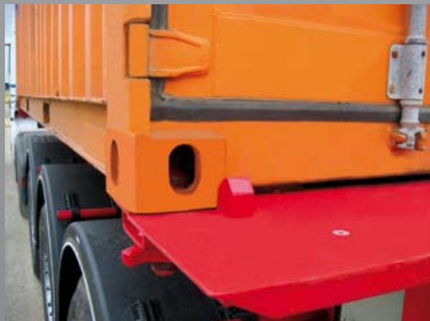
Discharge panel with integrated container lock
