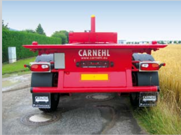
Protective panels at rear end
