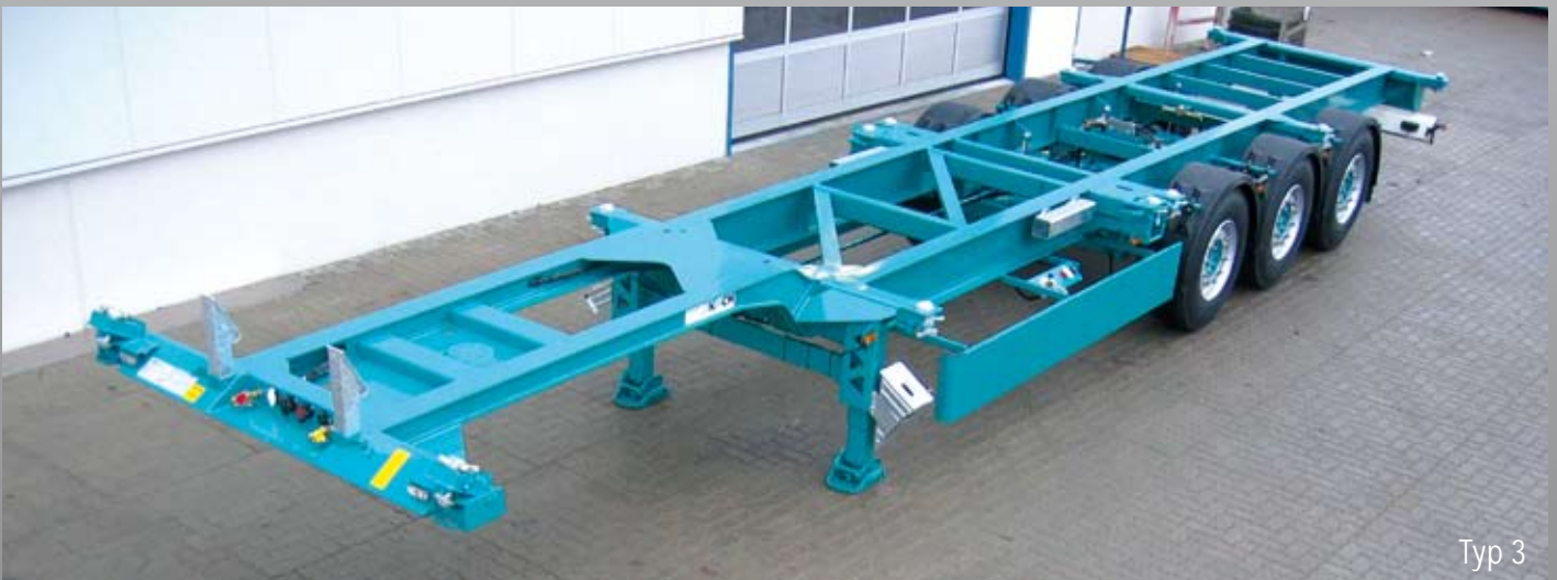
Container chassis type CCS/GF ,harbour
