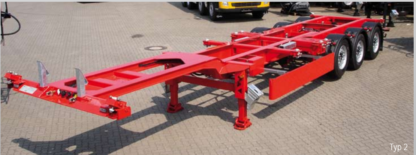
Container chassis type CCS/HS with rear telescopic extension
