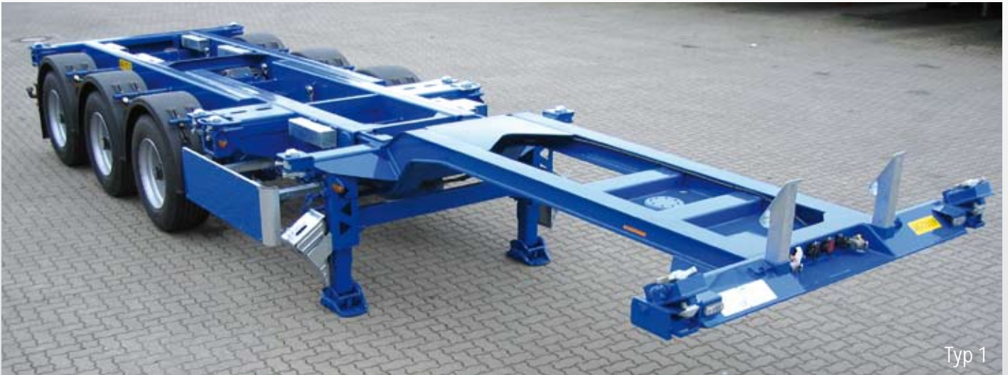
Container chassis type CCS/MHS with central and rear telescopic extension
